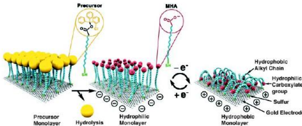
Fig. 1. Idealized representation of the transition between straight (hydrophilic) and bent (hydrophobic) molecular conformations (ions and solvent molecules are not shown). The precursor molecule MHA, characterized by a bulky end group and a thiol head group, was synthesized from MHA by introducing the (2-chlorophenyl)diphenylmethyl ester group.
