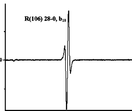
FIG. 4. Signal-to-noise ratio of R(106) 28-0, b_{10} sketched by our portable laser system. Time constant: 20 ms. Modulation width: 6 MHz.
