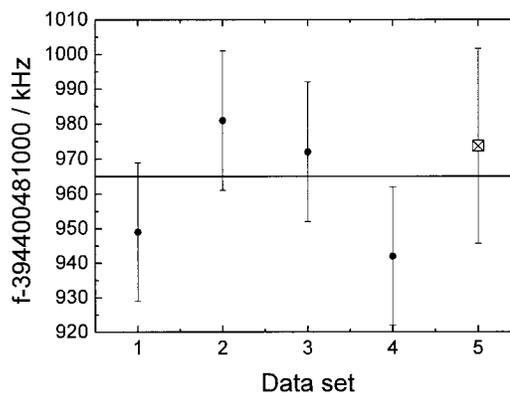
Fig. 5. Measured frequency of the  $^{87}\text{Rb}$   $F = 1-1$  two-photon transition within 40 days.
