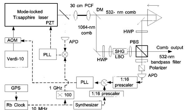
Fig. 1. Optical frequency comb system of the Center for Measurement Standards, Taiwan: DM, dichroic mirror; APDs, avalanche photodiodes; SHG, second-harmonic generation; AOM, acousto-optic modulator; PZT, piezoelectric transducer; PCF, photonic crystal fiber; HWP, half-wave plate; PLL, phase-locked loop; LBO, lithium triborate; GPS, global positioning system.
