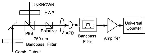
Fig. 2. Experimental setup for the beat note frequency measurement: PBS, polarizing beam splitter.
