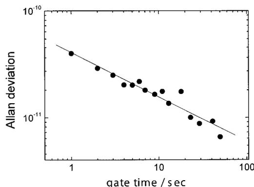
Fig. 4. Allan deviation of the beat frequency between our optical frequency comb and the Rb-stabilized laser.
