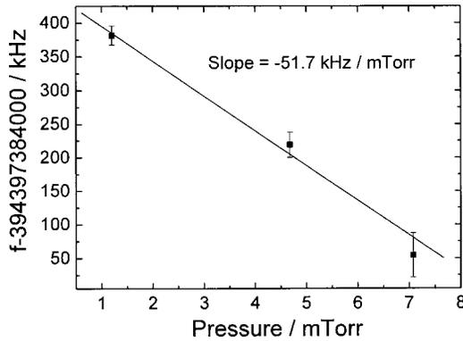
Fig. 6. Frequency shift of the two-photon line center versus the pressure in the Rb cell. The 760-nm laser is stabilized on the  $^{87}\text{Rb}$   $F = 2-2$  two-photon transition.
