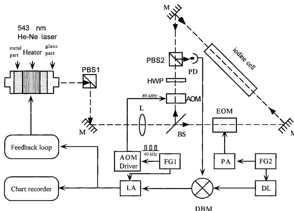
Fig. 1. Schematic diagram of our FM-stabilized laser system. PBS: polarizing beam splitter; M: mirror; AOM: acousto-optic modulator; EOM: electro-optic modulator; HWP: half-wave plate; L: lens; BS: beam splitter; PD: photo-diode; FG: function generator; PA: power amplifier; DL: delay line; LA: lock-in amplifier; DBM: double-balance mixer.
