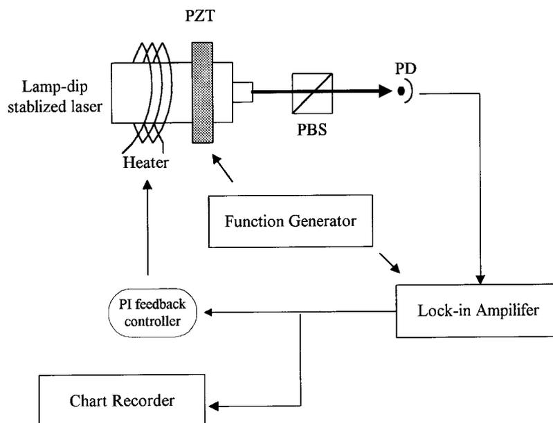
Fig. 5. Schematic diagram of the Lamb-dip stabilized laser system.
