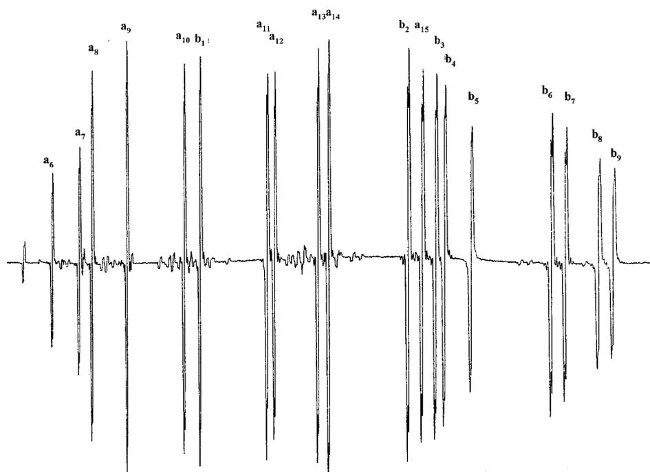
Fig. 3. FM hyperfine spectrum of the iodine at 543 nm. Here, the lock-in time constant is 100 ms and modulation frequency is 5 MHz. Note that there are weak lines among the main hyperfine lines. The frequency scale is not linear.
