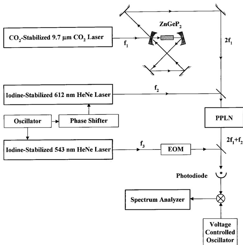
Fig. 8. Schematic diagram of the absolute frequency measurement of 543 nm iodine-stabilized HeNe laser. Here, EOM: electro-optic modulator; PPLN: periodically-poled LiNbO<sub>3</sub>.
