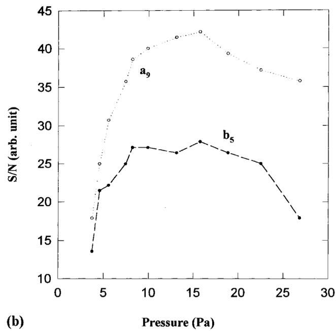
Fig. 2. The signal-to-noise ratio (S/N) vs. the iodine vapor pressure in our FM spectroscopy experiment for 120 cm iodine cell (a) and for 6 cm iodine cell (b).
