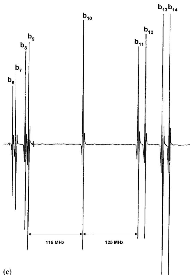
Fig. 4. (a) The hyperfine spectrum obtained by Melles Griot 05LGR024-S laser. The S/N of the  $a_9$  line is  $\sim 8000$  normalized to 1 Hz bandwidth. (b) The expanded view of the spectral range near  $a_9$  line (the recommended wavelength standard). Two crossover resonances are found near the  $a_9$  line. (c) The hyperfine spectrum obtained by Melles Griot 05LGR323 laser. The  $b_{10}$  line is far away from the neighboring main lines and crossover resonances.
