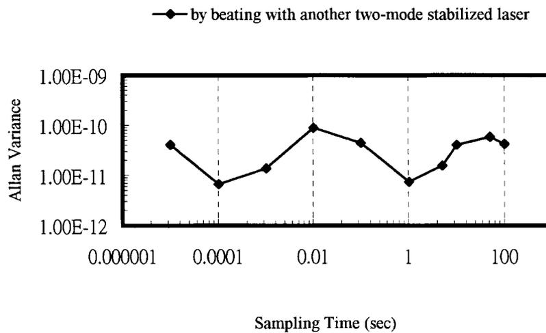
Fig. 7. Allan variance of the two-mode stabilized laser system.
