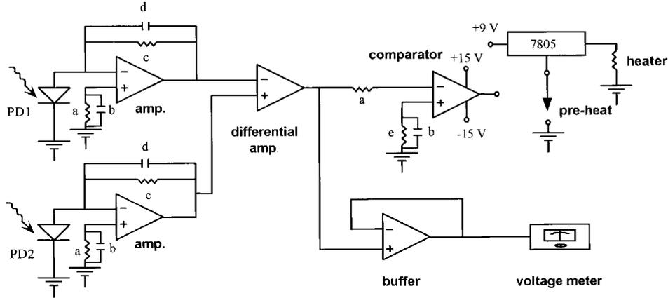
Fig. 6. The circuit of the bang-bang control. Here, a: 100 kΩ; b: 0.1 μF; c: 330 kΩ; d: 5 nF; e: 1 kΩ.
