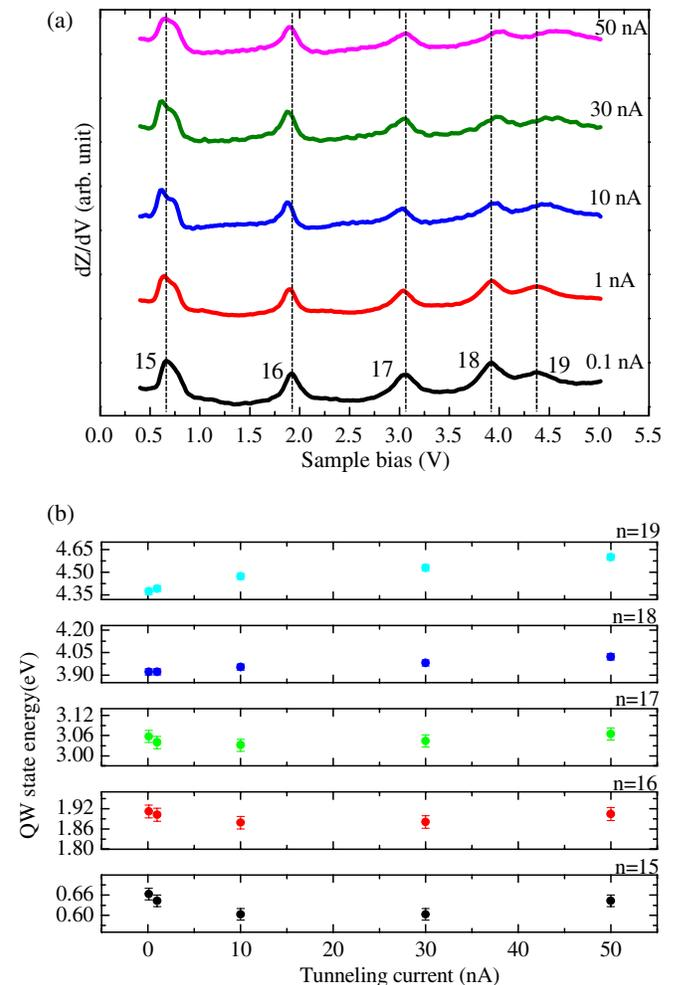
FIG. 2 (color online). (a)  $dZ/dV$ - $V$  spectra acquired on the island with a thickness of nine atomic layers at currents of 0.1, 1, 10, 30, and 50 nA. The peaks of quantum-well states in the spectrum are marked by quantum numbers. Dashed lines mark the peak energies at 0.1 nA.
