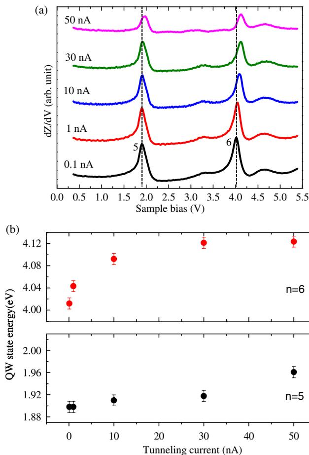
FIG. 1 (color online). (a)  $dZ/dV$ - $V$  spectra acquired on the island with a thickness of two atomic layers under set tunneling currents of 0.1, 1, 10, 30, and 50 nA. The peaks of quantum-well states in the spectrum are marked by quantum numbers 5 and 6. Dashed lines mark the peak energies at 0.1 nA. (b) The energies of two peaks as a function of tunneling current, showing a monotonically positive energy shift.
