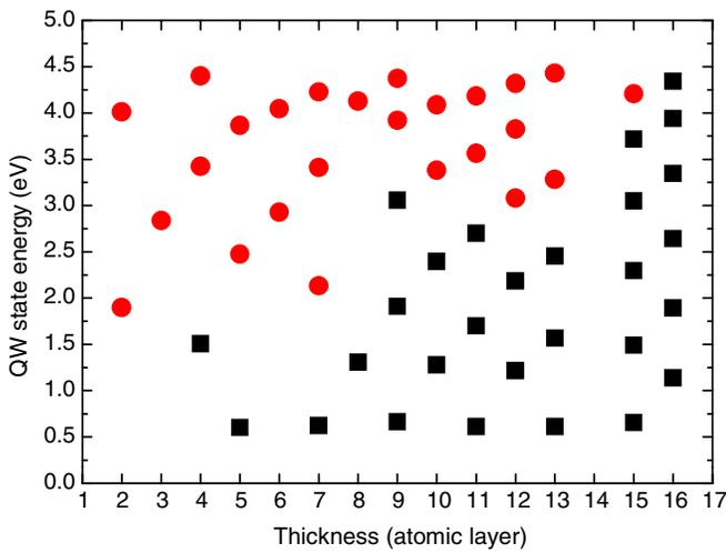
FIG. 3 (color online). Energies of quantum-well states at 0.1 nA versus island thickness. The energy shifts of quantum-well states behaving like the first (second) mode are marked by circles (squares).
