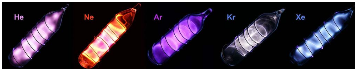
Fig. 13 Six gas discharge tubes are enclosed glass tubes filled with a gas at low pressure through which an electric current is passed. Electrons in the gaseous atoms first become excited, and then fall back to lower energy levels, emitting light of a distinctive color in the process. Shown are gas discharge tubes of helium, neon, argon, krypton, and xenon.
